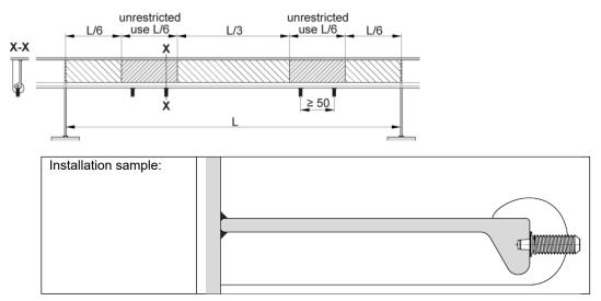
The X-BT fasteners may also be used in the restricted areas based on a case-by-case static investigation.
